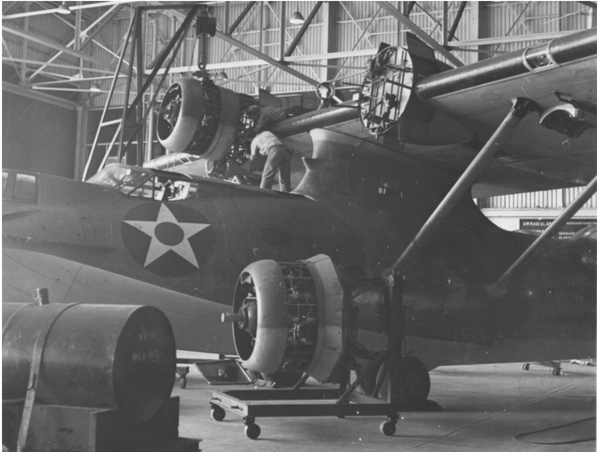
PBY-5 Catalina undergoes engine change at NAS Kaneohe Bay (Photo courtesy Cliff Dohrmann Collection)
